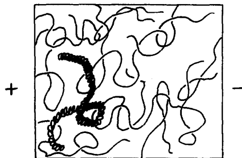
Fig. 3. A schematic representation of the entanglement coupling interaction of DNA, moving under the influence of an electric field, with the HEC molecules in the buffer.
